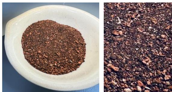
Figure 1. Ferrous sands - waste from alumina production
