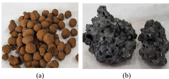
Figure 3. Iron ore pellets (a), iron ore agglomerate (b)
