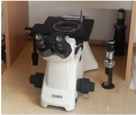
Figure 4. Metallographic inverted microscope METAM LV-32
