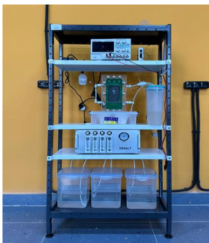
Figure 3. Bench installation for electro dialysis of \text{Na}_2\text{SO}_4 solutions
