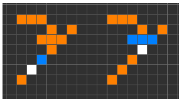
Figure 4 – Operation of OR-gate upon receiving input ‘01’.
