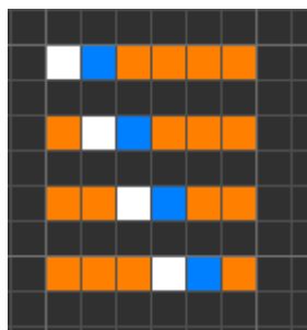
Figure 1 – Wires and moving electrons in Wireworld. From top to bottom: successive generations of a wire with one moving electron.
