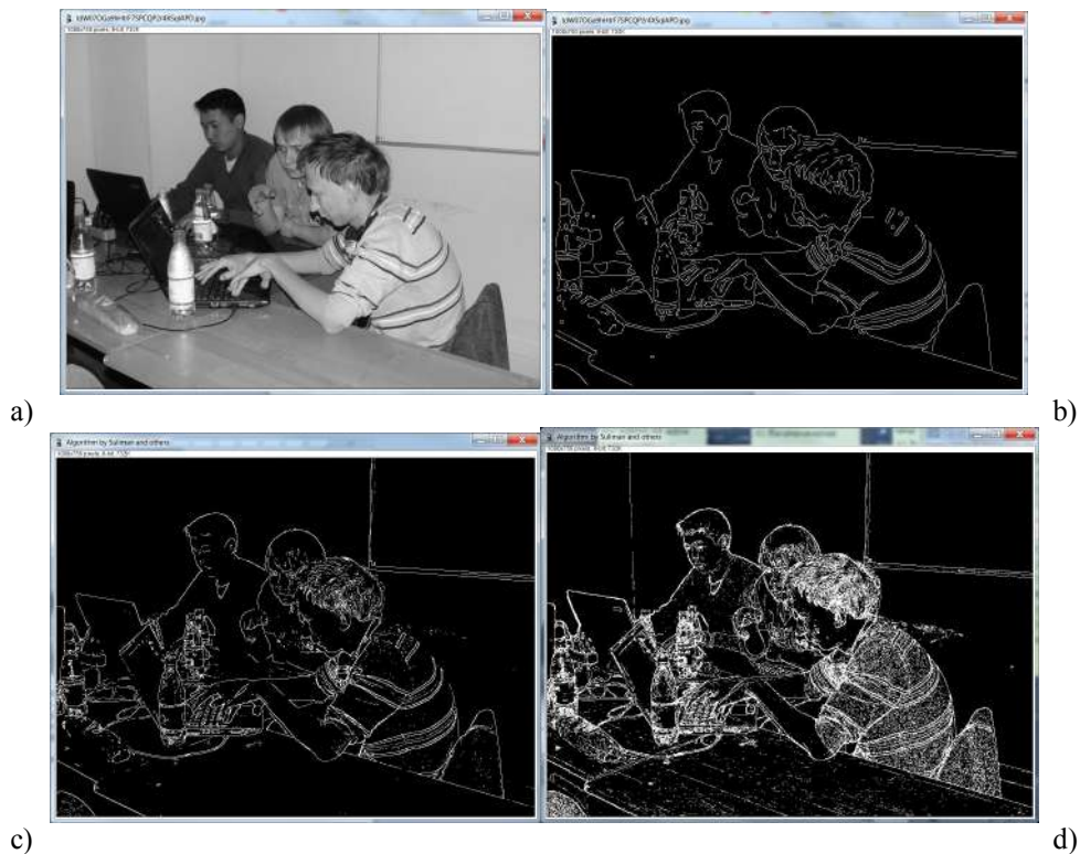
Figure 6. a) original image, b) edges detected by Canny edge detector with default parameters, c) edges detected by developed plugin with default parameters, d) edges detected by developed plugin with parameters “Low value” = 0, “High value” = 20, “Weight” = 256
