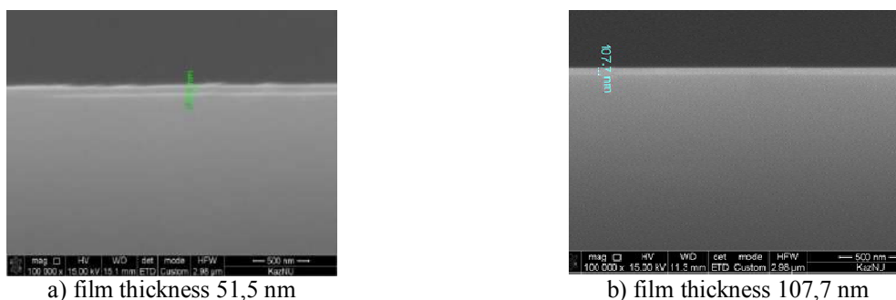
Figure 1. SEM-image of the cleavage c-Si/a-C:H films structure
