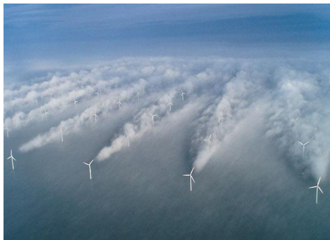
Fig. 2. Turbulent trace of propeller-type wind turbines
