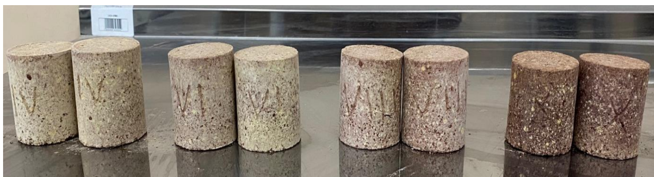
Figure 6. General view of samples with the addition of diatomite after firing at 1100 °C x 1 hour
