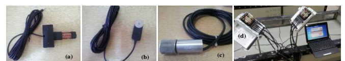
Figure 22. Sensors and data logger (a) Decagon 5TM moisture and temperature sensor (b) Decagon MPS-1 dielectric water potential (suction) sensor (c) Apogee SO-100 & 200 Series oxygen sensor (d) Decagon Em50 Datalogger Decagon DataTrac3 Software
