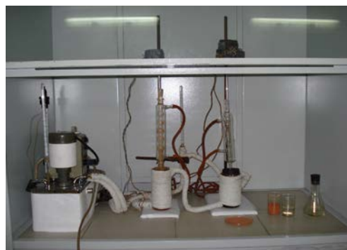
Figure 1. Laboratory Setup for Acid Decomposition of Krasnooktyabr Bauxite
