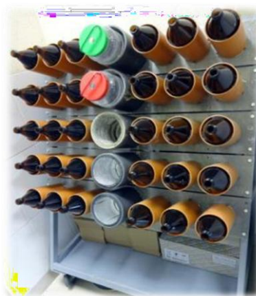
Figure 1. Laboratory stand for conducting study on agitated leaching
